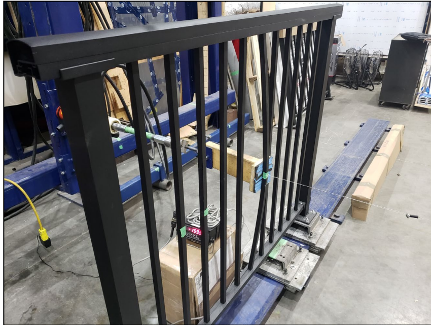
Figure 1. 2015 NBC, Section 4.1.5.14, Clause (3): In-Fill Load Test
